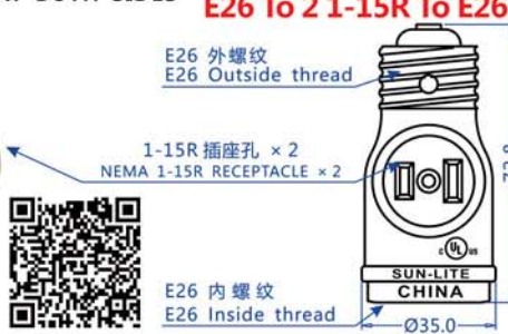
E26 转接灯座, 及双侧 NEMA 1-15R 极性插座 E26 LAMPHOLDER, BASE EXTENSION WITH NEMA 1-15R RECEPTACLES AT BOTH SIDES
