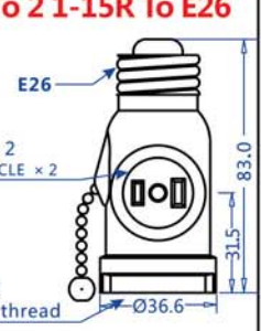
E26 转接灯座, 及双侧 NEMA 1-15R 极性插座 E26 LAMPHOLDER, BASE EXTENSION WITH NEMA 1-15R RECEPTACLES AT BOTH SIDES
